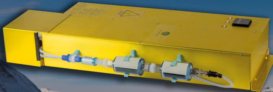
*The CON 765 NO<sub>y</sub> converter was developed for combination with a highly sensitive ECO PHYSICS chemiluminescence analyzer and allows the measurement of the total reactive nitrogen oxides (NO<sub>y</sub>) in the range of parts per trillion.*
