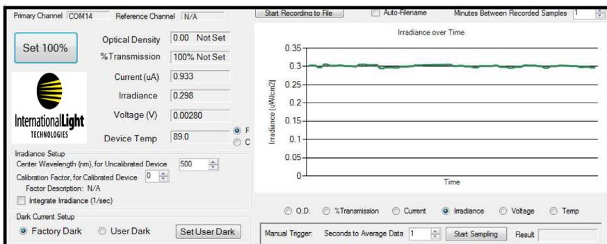
**TREND** - Records all 6 parameters while displaying the trend over time for the user switchable parameter. Multiple examples of trend can be run simultaneously to allow multi-unit comparisons. Trend also has a user-friendly calibration feature.
