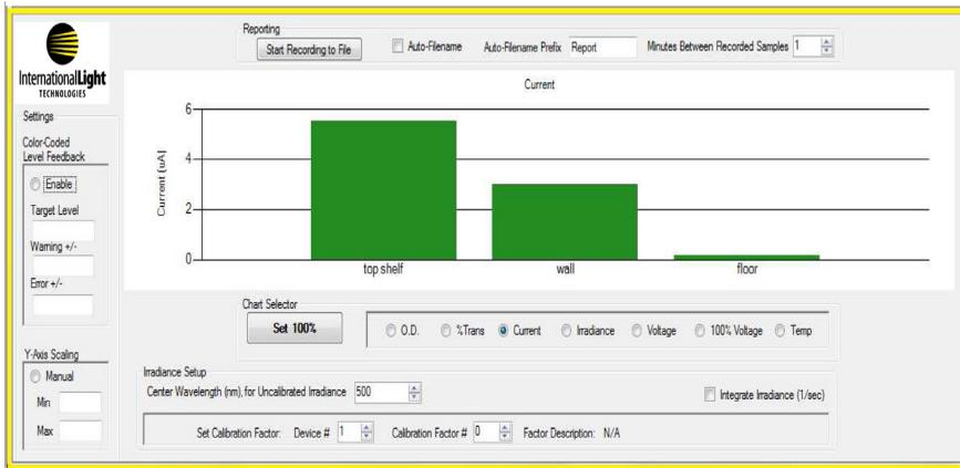
**BAR** - Allows multisystem, datalogging and displays the user switchable parameter in a bar graph. The expandable graph can accommodate up to 32 systems simultaneously with use of hub(s). User can enter nicknames for each unit to define the location, application, version, serial number, etc. Customer can program max and min warning levels and use color coded bar responses for easy troubleshooting.
