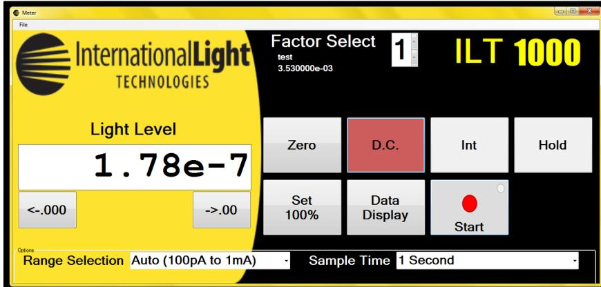
**Meters** - Designed to maintain the look and feel of the Industry Standard ILT1700 Research Radiometer. Designed for wireless use with windows 8 tablets and touch screen computers, the larger, user-friendly panel includes buttons for hold, zero, integrate, factor, range, average and units selection.
